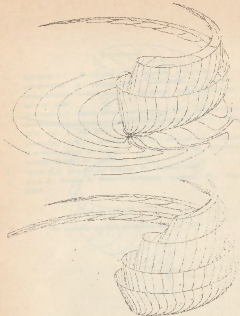
Figs 9-10 The whole system of field lines in the space can be represented as a set of field-line systems on surfaces one enclosed in another. Near the charge it is a system of cones one enclosed in another, on which straight field lines are lying. In Figs 9.10 the surfaces from Figs 4 and 6 and 4.6-8, respectively, are enclosed one in the other.
